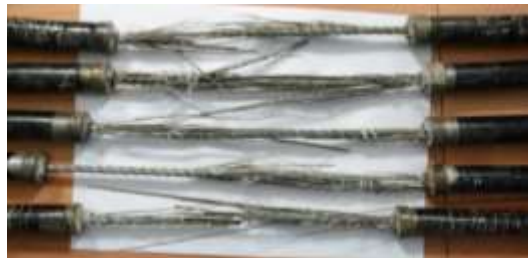
Fig. 6 Failure of tensile specimens
