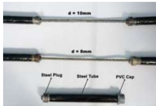
Fig. 1 Details of the tensile specimens
